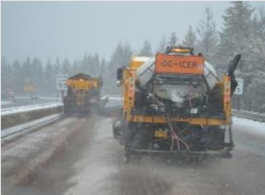
Corrosion inhibited liquid magnesium chloride (1990s)
