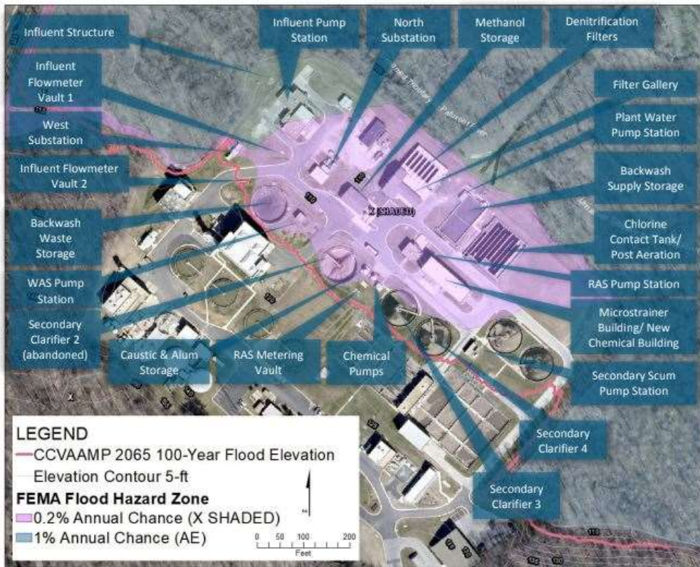
Figure 4-2. Floodplain at Parkway Wastewater Treatment Plant
