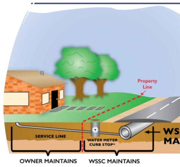
"Curb Stops" are used when the Water Meter is located inside the home.
