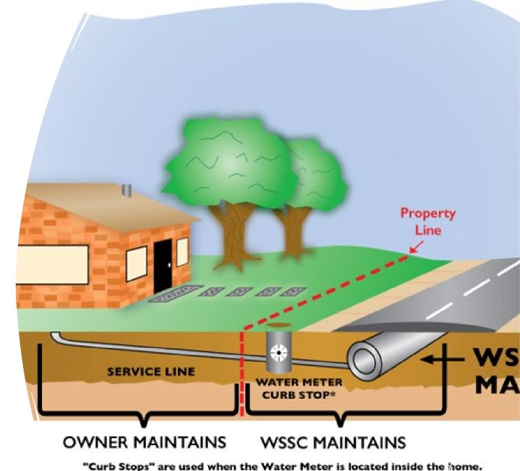
"Curb Stops" are used when the Water Meter is located inside the home.
