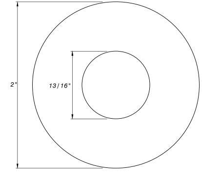
MATERIAL: LOW ALLOY STEEL IN ACCORDANCE WITH ASTM A307, LATEST REVISION THICKNESS:1/4"
